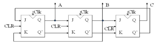
a) Suppose the flip-flops are reset initially, enumerate the states (A,B,C) according to the clock sequence. Fill the following table.
