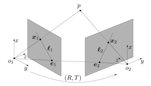
Since the cameras are calibrated, we have  $K_1 = K_2 = I$ . The cameras are centered at  $o_1$  and  $o_2$ , respectively. The homogeneous vectors  $\mathbf{e}_1$  and  $\mathbf{e}_2$  are the *epipoles*, and can be intuitively thought of as any of the following:
