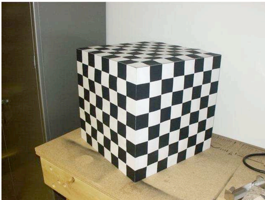
Figure 2. Cube-shaped calibration rig (from MaSKS).
