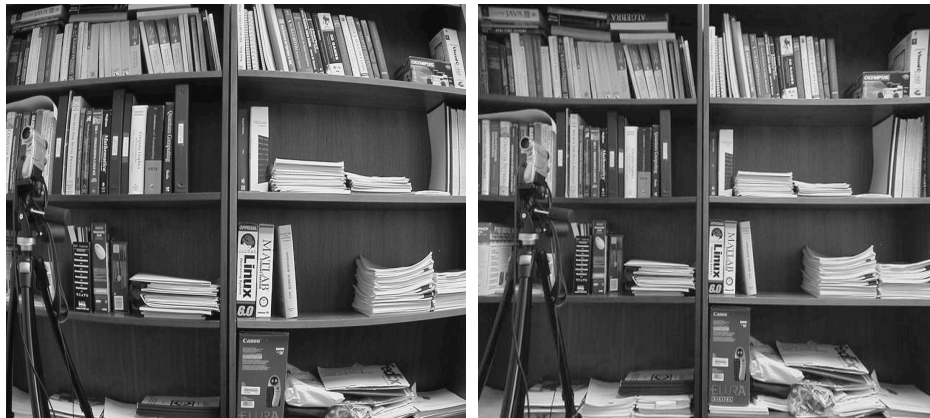
Figure 1. Example of radially distorted image (left) and its rectified version (right). (From MaSKS)
