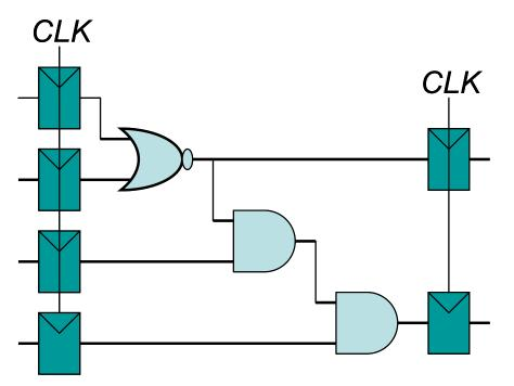
a) If there is no clock skew, what is the maximum operating frequency of this circuit?
