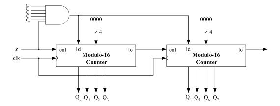
IV(2). Design a counter with a repeated output sequence 15, 0, 1, 2, 8, 9, 10, 6, 7, with a modulo-16 counter and a minimal combinational network. Write the Boolean expression and draw the schematic diagram.
