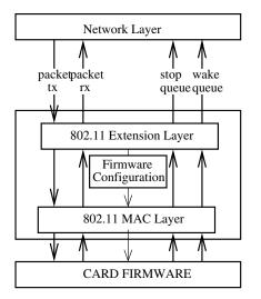
Fig. 2. Implementation of the  $2\frac{1}{2}$ -stage stage pipeline architecture within existing 802.11 based wireless cards.
