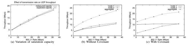
Fig. 6. Variation of aggregate bandwidth of two nodes with unequal transmit rates. In the subfigure (a), node 2 is configured to operate at 36 Mbps, while node 1 varies from 6 to 36 Mbps. Without Covenant, we can see that node 1 operating at lower rates affects the aggregate throughput achieved significantly. In the subfigure (b), we use Covenant to ensure that we split the bandwidth using air-time instead of channel access fairness provided by regular 802.11.
