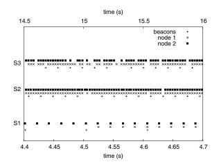
Fig. 4. Timeline of load exchange packets and beacons. There are three different snapshots (S1, S2 and S3) each showing the beacon arrival times, node 1 load exchange packet arrival times and node 2 load exchange packet arrival times. The top two snapshots use a different scale of timeline.
