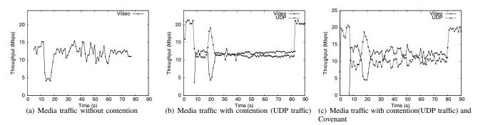
Fig. 7. In this experiment, we study the effect of Covenant on a media stream with and without contention from other UDP traffic generators. The media node is configured to obtain at least 3 times the bandwidth received by another node.
